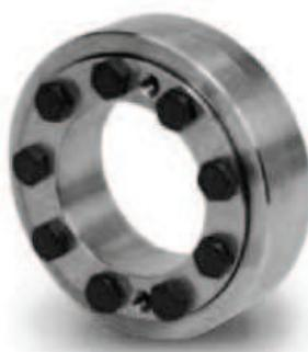
No need for a Torque Wrench with these Clamping elements, just tighten the screws in clockwise sequence in stages until the front faces of the flange and outer ring are aligned. This allows the transmission of torque values shown in the table. This overcomes the problems often encountered where units are either under or over tightened causing failures in transmission. There can also be a time saving in that powered tools can be used for the belt tightening.
