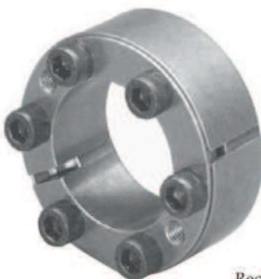
These clamping elements provide good torque transmission from a compact, low cost assembly. These units must always be installed inside the hub, and will then provide a reasonable level of concentricity. A small axial movement of the hub occurs during clamping.
